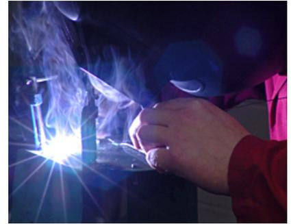
TIG welding requires a gas shield protection of pure(Argon). In MMA mode, it allows you to weld with any kind of electrodes: rutile, basic, stainless steel or cast iron.
